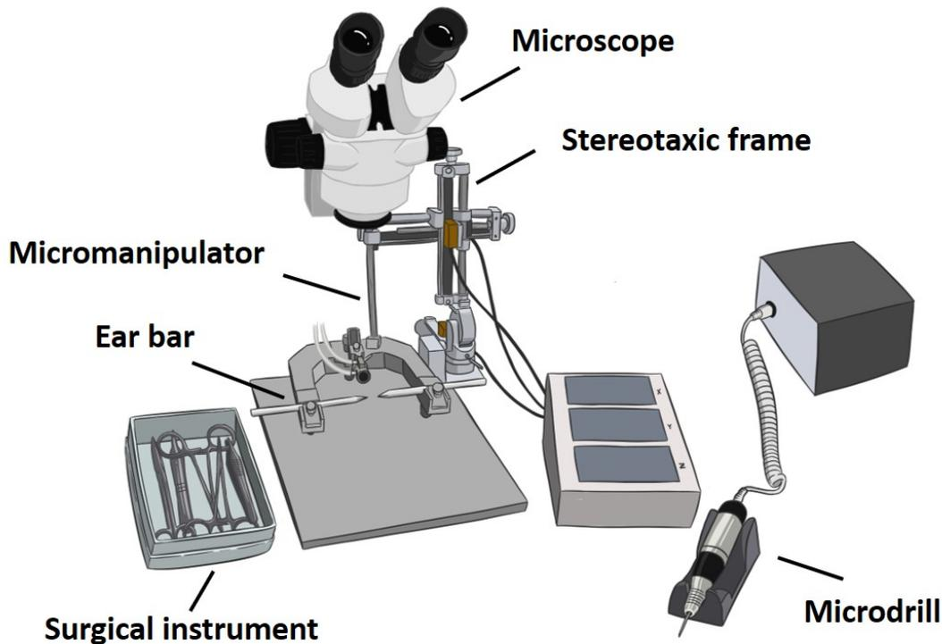
**Stereotaxic frame, auxiliary ear bar, and micromanipulator**
